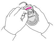
Turn the ring a very short distance, until it stops. When the recessed area on the ring is *not* lined up with the recessed area surrounding the ring, the mouse is locked.
